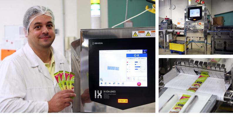
The touchscreen on the machine immediately provides information on the nature of the foreign bodies and exactly where in the product they are hiding.
