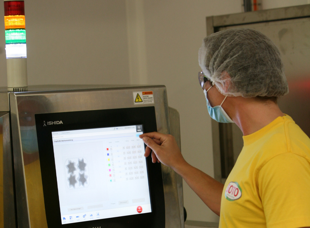
product particle trapped in sealing area spotted by Ishida X-ray system
