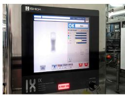
Although we record very few rejects (approx. 7 out of 100,000 bottles), the presence of the Ishida side beam X-ray inspection system allows us to offer our customers extra evidence of our production quality.
